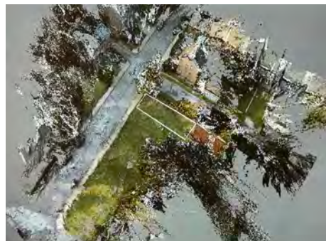
Point cloud image of the site and surrounding context for RE_ CON 01 collected using terrestrial LiDAR scanning.
